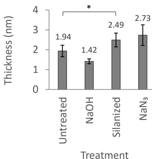
**Figure 1** Average surface film thickness of silicon wafers upon consecutive chemical treatments in the order shown above. \*Significant different, one-way ANOVA and Tukey's HSD test,  $p < 0.05$ ,  $n = 26$ . Error bars are the standard deviations.
